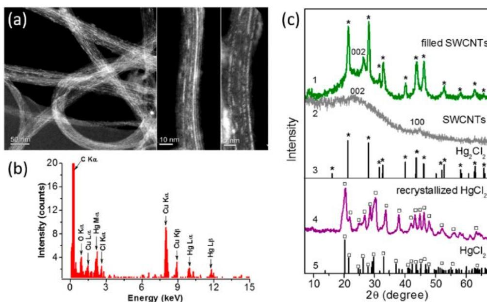
Figure 1. (a) HAADF/STEM images and (b) EDX spectrum of filled SWCNTs. (c) XRD patterns of filled (1) and initial SWCNTs (2), polycrystalline  $\text{Hg}_2\text{Cl}_2$  (3), mercury chloride recrystallized without addition of SWCNTs (4), and polycrystalline  $\text{HgCl}_2$  (5).
