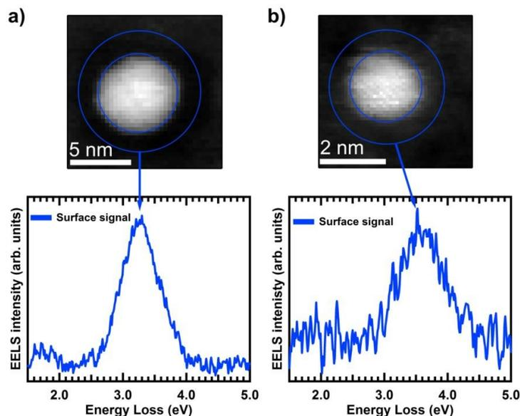
**Figure 1.** a) STEM-HAADF image of a 6.5 nm particle embedded in silica and the EEL spectrum associated to the surface b) STEM-HAADF image of a 2.0 nm particle embedded in silica and their EEL spectrum associated to the surface.
