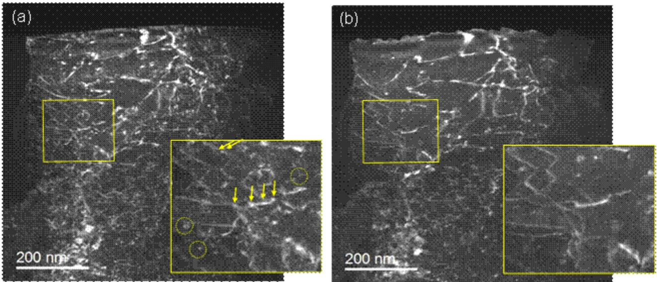
Fig. 2 Weak-beam STEM images of steel sample before annealing (a) and after 30 min (b) from the time when temperature reaches 400°C. Insets are magnified images of the areas denoted in (a) and (b). Some of dislocations as shown in inset image of (a) are disappeared after 30 min.
