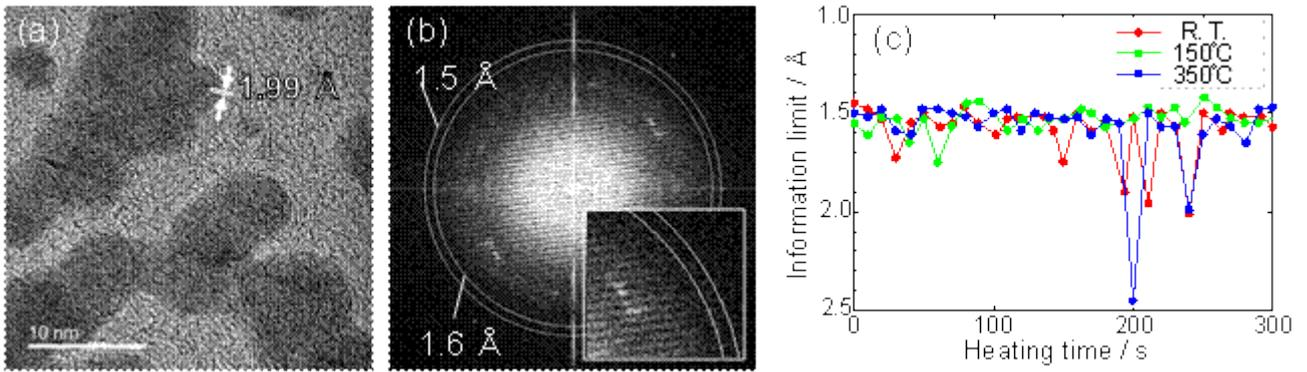
Fig. 1 AC-TEM image of Au/Pd grating (a) and Young fringe pattern(b) at 350°C. (c) is the heating time dependence of information limit of the grating sample at room temperature, 150°C and 350°C.
