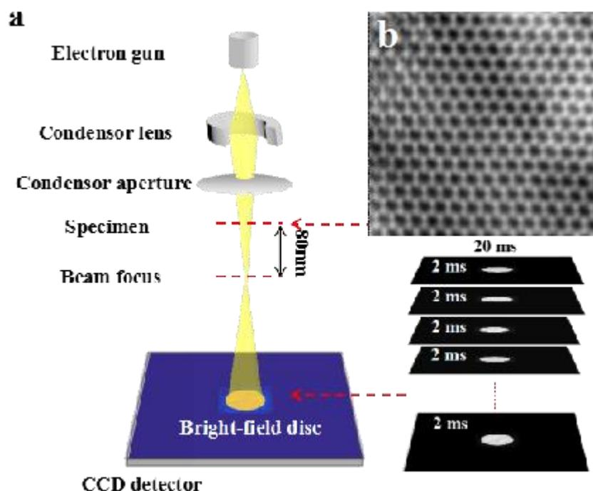
**Figure 1.** (a) Schematic of (a) the experimental configuration used for ptychographic reconstruction and (b) Ptychographical reconstruction of a MoS<sub>2</sub> monolayer oriented along a <001> direction.
