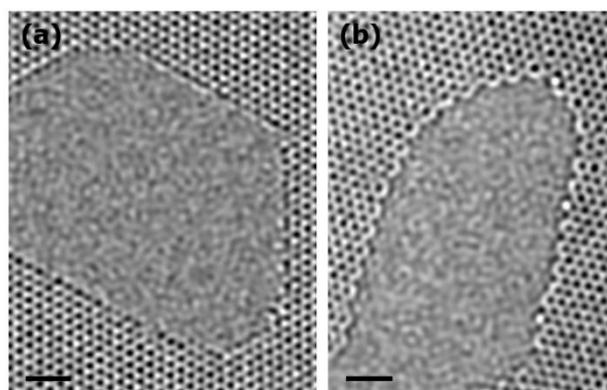
Fig 1. TEM images of nanopores fabricated at room temperature with zigzag edges (a) and at 600°C with armchair edges (b). The scale bars are 1 nm.
