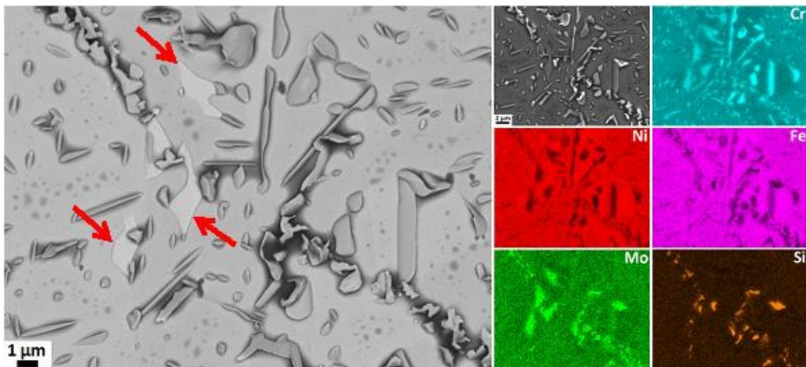
Figure 2 - BSE-SEM image of Alloy 33 after isothermally aging at 800 °C for 100h. Electrolytic polishing/etched.
