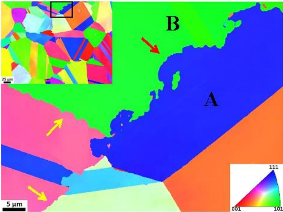
Figure 1 - EBSD maps of Alloy 33 after isothermally aging at 800 °C for 5h.
