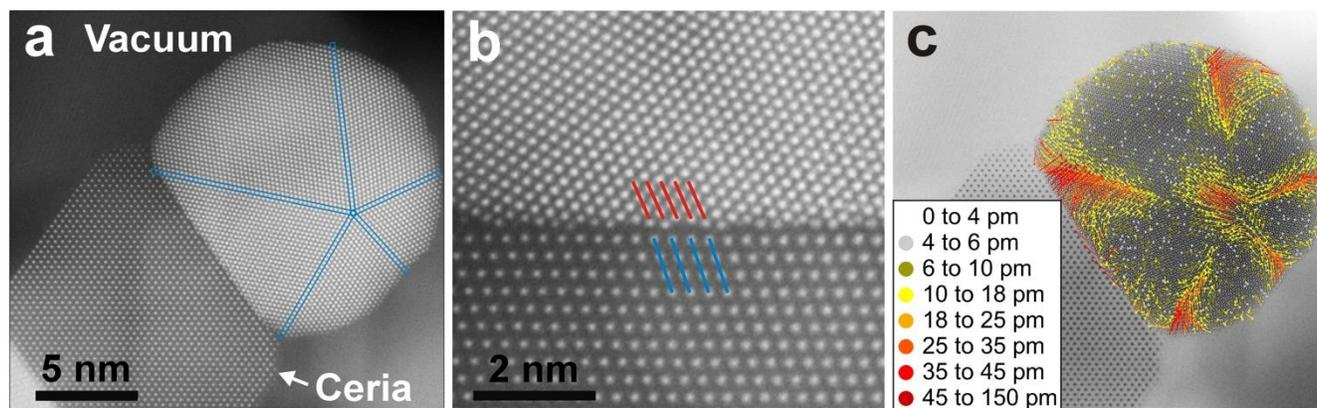
**Figure 1.** (a) High-precision side-view HAADF STEM image of a ceria-supported Pt NP in the [110] zone axis. Blue rectangles mark the five {111} twin boundaries separating the grains of the decahedron NP structure. (b) Enlarged image of the NP-support interface region in (a) with {111} planes marked on either side of the interface to reveal the presence of an interface dislocation. (c) Atomic column displacement map showing the direction and magnitude of lattice deformations.
