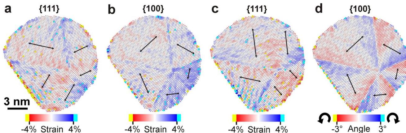
**Figure 2.** (a-c) Local strain maps and (d) angle map for the labeled crystallographic planes that are marked by black arrows. Red signifies compressive strain and CCW angle rotation. Blue signifies expansive strain and CW angle rotation. Bright yellow and light blue signify large values off the figure color scale.
