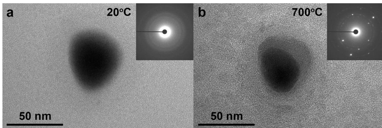
**Fig. 2** (a,b) BF TEM images on individual Fe NP at (a)  $20^\circ\text{C}$ ; and after *in situ* heating to (b)  $700^\circ\text{C}$ . The associated SAED patterns (inset) show an increase in crystallinity from (a) diffuse diffraction rings; to (b) additional well-defined diffraction spots.
