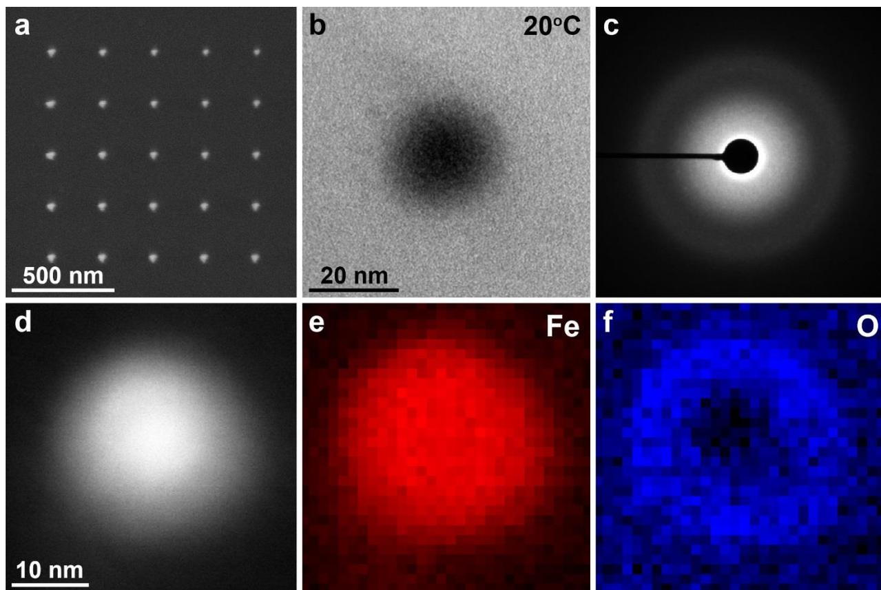
**Fig. 1** (a) SEM image of an array of Fe NPs produced by FEBID, ranging from  $\sim 20$  nm to  $\sim 50$  nm in diameter. (b) BF TEM image of an individual Fe NPs ( $\sim 20$  nm in diameter) at  $20^\circ\text{C}$ ; and (c) corresponding SAED pattern from the Fe NP in (b) displaying diffuse diffraction rings. (d) Scanning TEM image of an individual Fe NP; and (e,f) EELS chemical maps showing its elemental distribution of (e) Fe; and (f) oxygen content.
