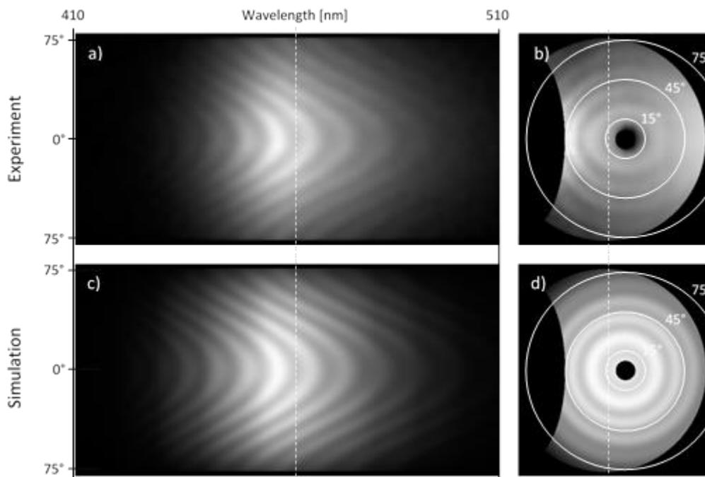
**Figure 2.** Slices extracted for the reconstructed 3D energy-momentum CL spectrum of InGaN multi-quantum wells in GaN film demonstrating strong angular dependence of the wavelength distribution: a) and c) are momentum-filtered energy spectra through the reconstruction at position indicated with the dotted line in b) and d); b) and d) are energy-filtered momentum spectra from the same data sets respectively displaying the angular distribution of light of wavelength at  $\sim 462$  nm.
