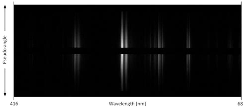
**Figure 1.** Energy-resolved momentum spectrum from a phosphor particle collected in a cathodoluminescence (CL) experimental setup. The angular distribution exhibits isotropic color (wavelength invariance) at all angles.
