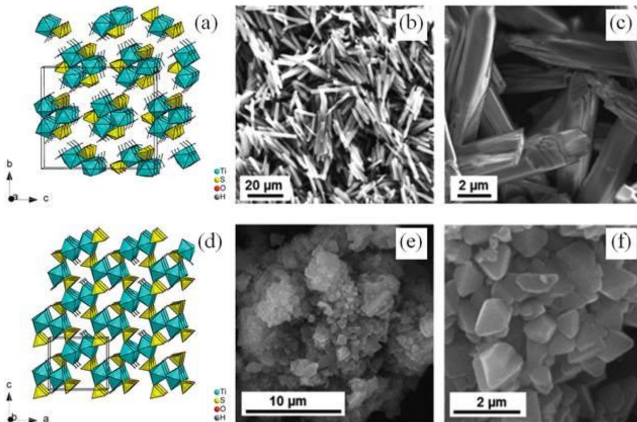
**Figure 1.** Structure of titanyl sulfate dihydrate (a) and titanyl sulfate monohydrate (d), and the corresponding metatitanic acid pseudomorphs (after titanyl sulfate dihydrate - b,c, and after titanyl sulfate monohydrate - e,f).
