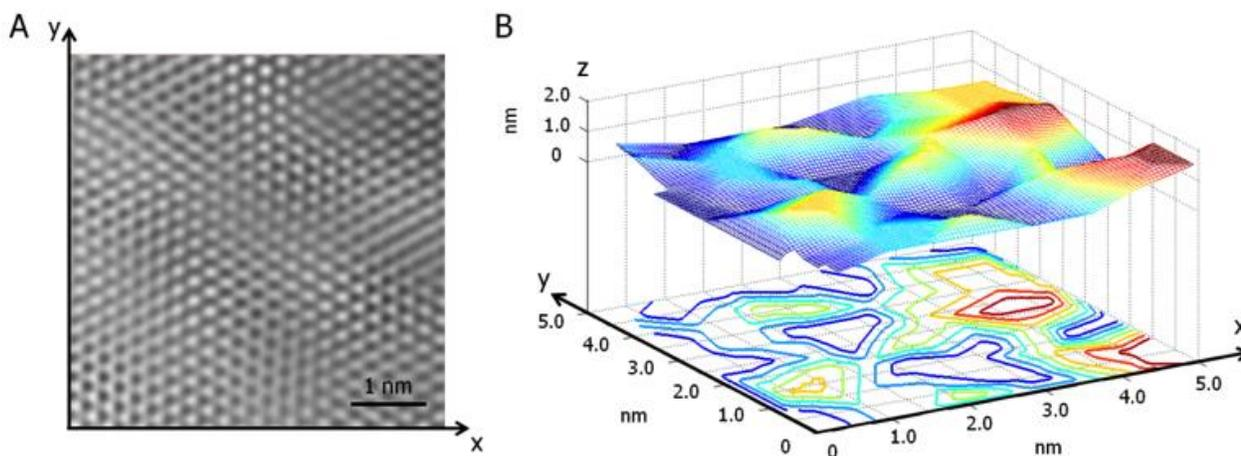
Figure 1. A: Filtered 2D TEM image of free-standing monolayer graphene
