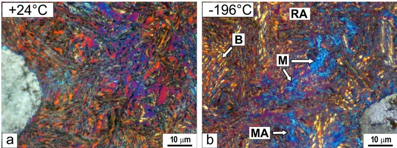
**Fig. 2** The ADI 400 microstructure revealed by heat tinting: a) room temperature, b) -196°C (RA - retained austenite, MA - metastable austenite, B - bainite, M - martensite)
