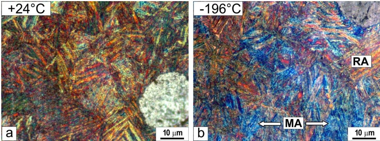
**Fig. 1** The ADI 300 microstructure revealed by heat tinting: a) room temperature, b) -196°C (RA - retained austenite, MA - metastable austenite)
