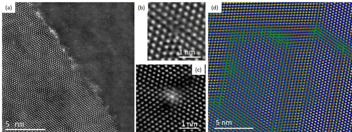
Fig. 2. (a) Annular dark field (ADF) STEM image of a SiC grain boundary showing the presence of isolated metallic fission product atoms along the boundary. (b) Atomic resolution image of an unoccupied Lomer-Cottrell dislocation in a SiC grain. (c) Atomic resolution image of a fission product atom present within a dislocation core in the SiC. (d) Atomic resolution false colour image showing the annihilation and termination points of stacking faults planes within a SiC grain.
