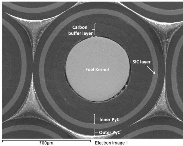
Fig 1. Secondary electron (SE) scanning electron microscope (SEM) image of a polished TRISO particle showing the various coating layers.
