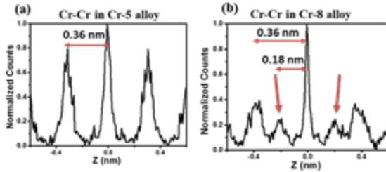
**Fig. 2:** Spatial distribution map obtained along successive (100) planes in  $\gamma'$  phase for (a) Cr-5 and (b) Cr-8 alloy.
