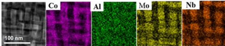
**Fig. 1:** Elemental mapping for the peak aged Co-10Al-5Mo-2Nb alloy in a scanning transmission electron microscopy (STEM) nano probe mode [2].
