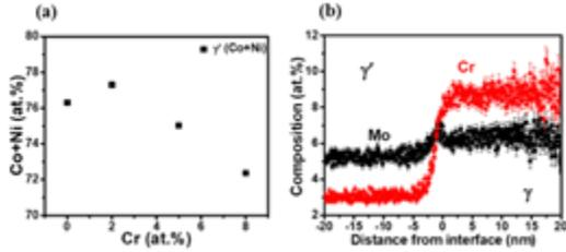
**Fig. 3:** Plot showing variation in Co + Ni concentration in  $\gamma$  phase with Cr addition to Co-30Ni-10Al-5Mo-2Ta-2Ti alloy. (b) Concentration plot showing distribution of Cr and Mo concentration across the  $\gamma/\gamma'$  interface for Cr-5 alloy aged at 900 °C for 50h.
