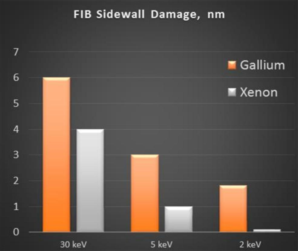
**Chart 1.** FIB sidewall damage in aluminium 6061 T6 at various accelerating voltages.
