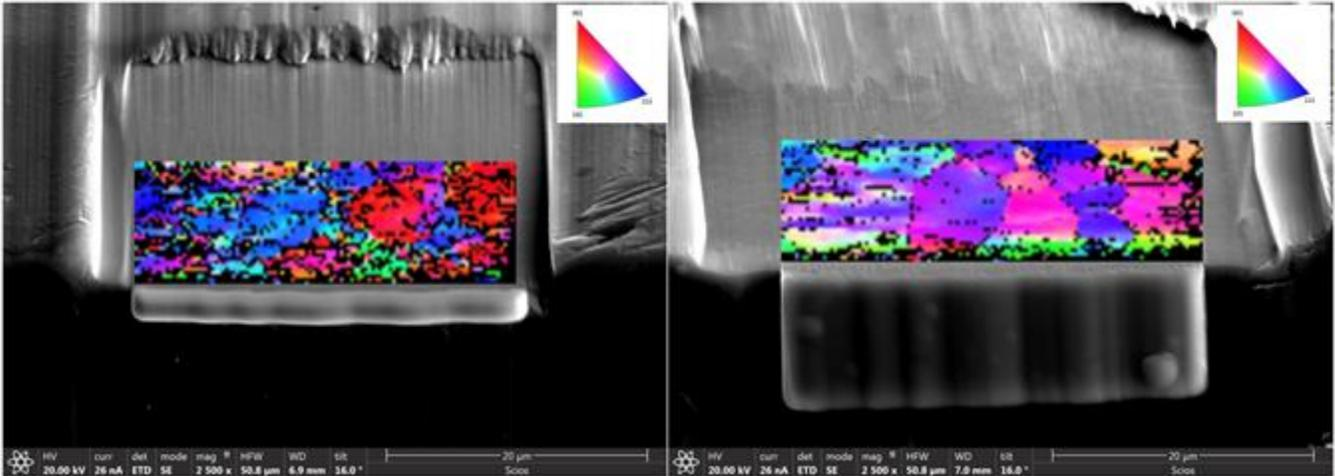
**Figure 1.** Inverse pole figure results of aluminium 6061 T6 with Ga<sup>+</sup> prepared surface (left) and Xe<sup>+</sup> prepared surface (right).
