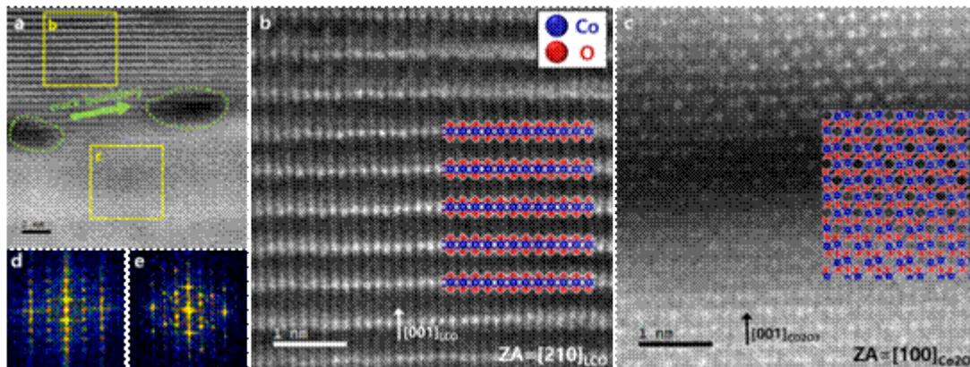
Figure 2. Atomic-scale resolution annular dark-field STEM image of overcharged  $\text{LiCoO}_2$ . (a) Different phases are separated by crack boundary. Detailed image of upper region and lower region of (a) are shown in (b) and (c), respectively. (d, e) FFT patterns which agree with the atomic structure drawn in (b) and (c). Unlike the layered structure ( $\text{Li}_x\text{CoO}_2$ ) shown in (b), (c) indicates newly induced cobalt oxide phase ( $\text{Co}_2\text{O}_3$ ).
