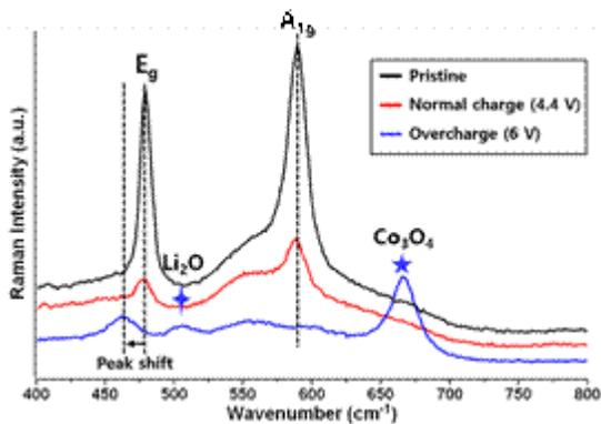
Figure 3. Raman spectra of  $\text{LiCoO}_2$  particles at different charge conditions. The pristine particle shows two distinct peak in  $E_g$  ( $479\text{ cm}^{-1}$ , O-Co-O bending) and  $A_{1g}$  ( $589\text{ cm}^{-1}$ , Co-O stretching). Contrastively, after overcharging, main bands weakening with peak shift of  $E_g \sim 461\text{ cm}^{-1}$  and newly induced peaks (i.e.  $\text{Li}_2\text{O}$  and  $\text{Co}_3\text{O}_4$ ) are shown.
