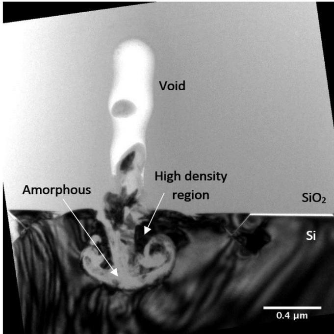
Figure 2. BF TEM of a microexplosion induced at the interface between Si and SiO<sub>2</sub>. A void is visible extending from the interface up into the SiO<sub>2</sub>. To either side within the Si is a highly compressed region containing high density crystalline phases.
