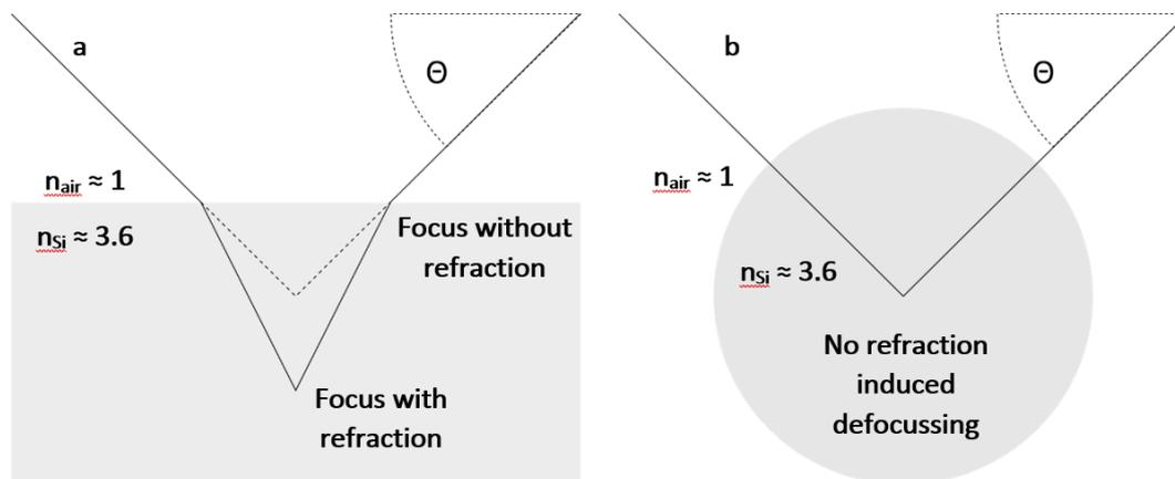
Figure 1. Ray diagrams of a focussed laser entering Si where for a flat surface (a) refraction causes a defocussing effect and for a sphere (b) no defocussing occurs allowing intensity dependant absorption to be more restricted to the focal point.
