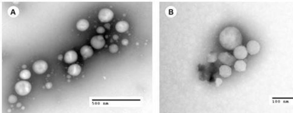
Figure 1: TEM of gelled soybean oil nanoparticles (A) and (B)
