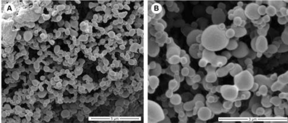
*Figure 2: Cryo-MEB observation of a colloidal hydrogel after sublimation (A) and a detail (B)*
