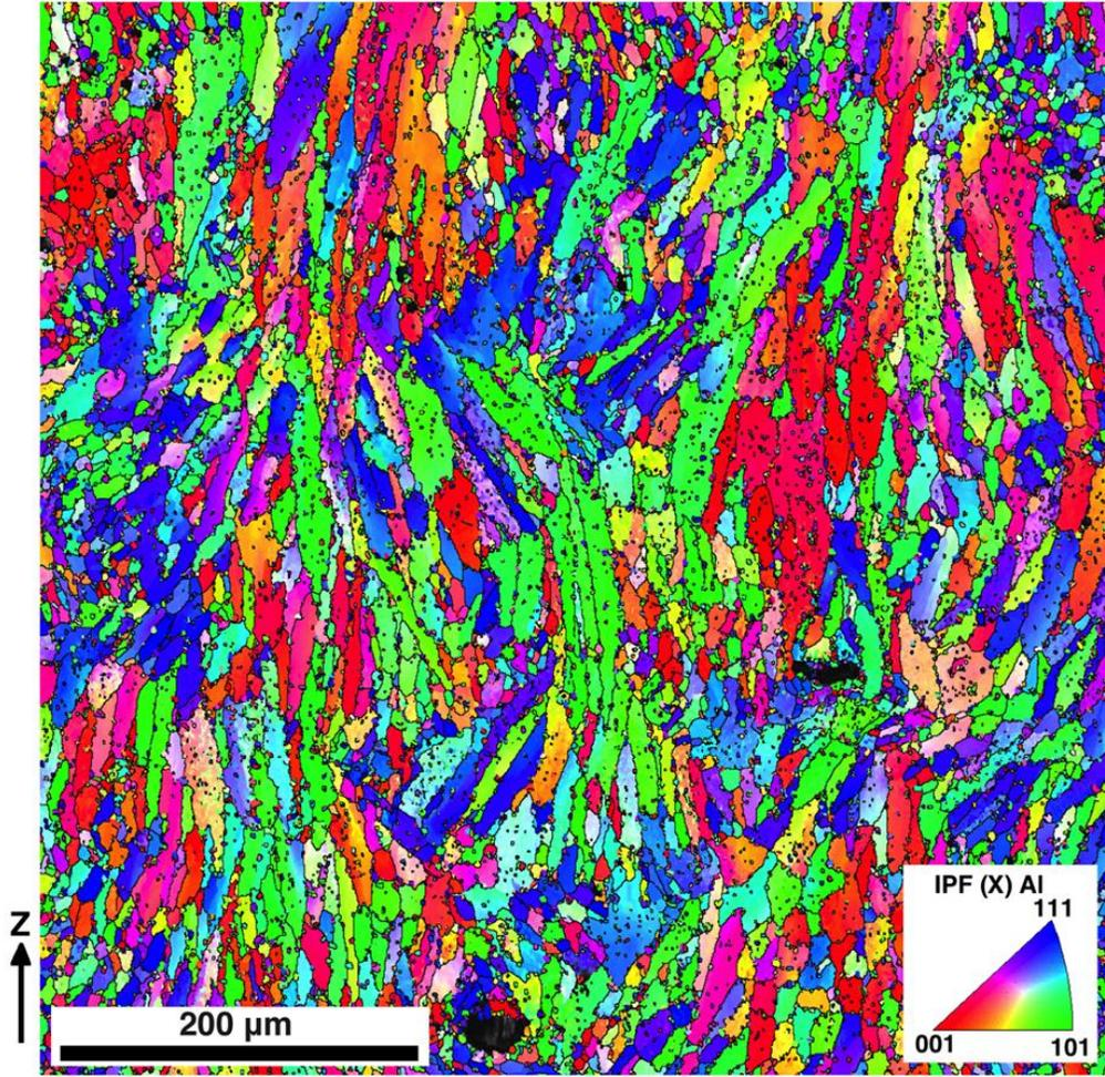
**Figure 1:** Inverse pole figure map of the AlSi10Mg aluminium alloy produced via selective laser melting after T6 heat treatment. The z-direction indicates the direction normal to the printing plane.
