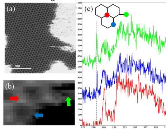
Fig. 2 (a) STEM-ADF image of a mono-layer graphene (b) STEM-ADF image of a mono-layer graphen edge (c) EELS spectrum obtained from each carbon atom
