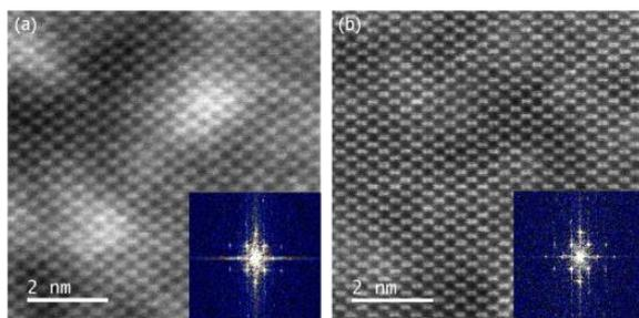
Fig. 1 STEM-ADF image of Si [110] by changing energy spread of electron at 30kV(a) 0.4eV, (b) 0.3eV)
