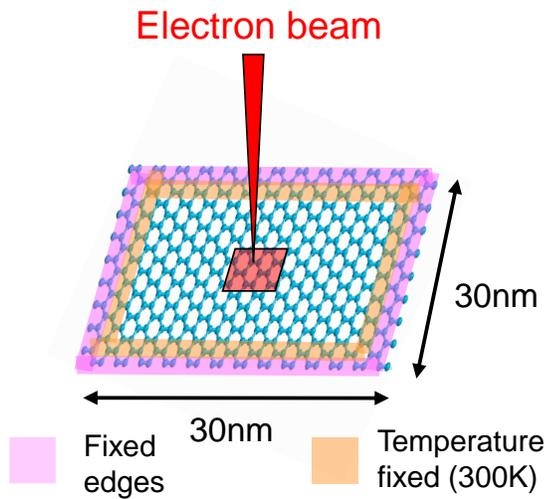
Fig. 1 Configuration of heating simulation in electron irradiated square-shaped graphene.
