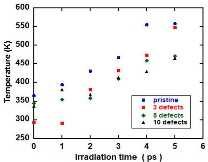
Fig. 4 Temperature of defective graphene nanoribbon as a function of electron irradiation time.
