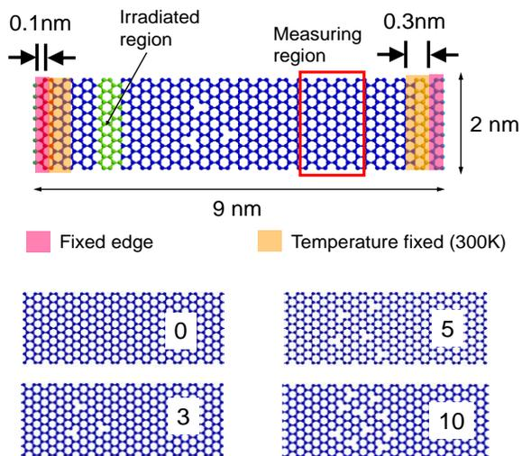
Fig. 3 Configuration of thermal transport simulation in electron irradiated graphene with mono-vacancy defects.
