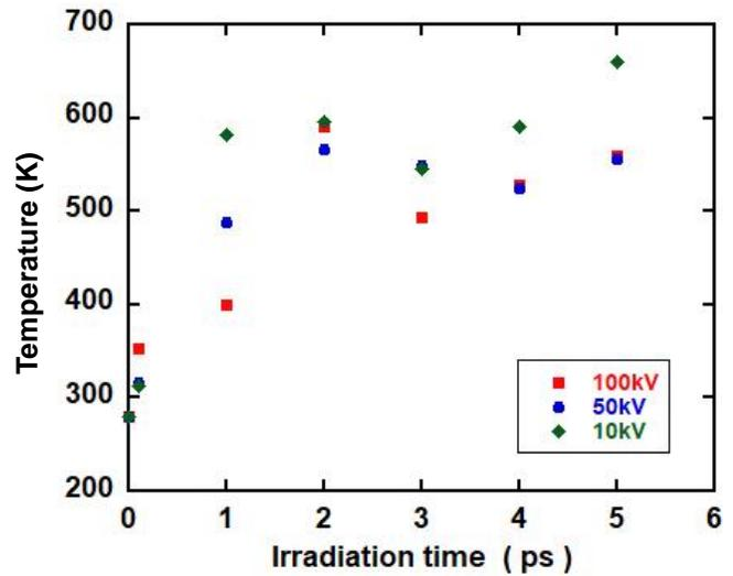
Fig. 2 Temperature of square-shaped graphene as a function of electron irradiation time.
