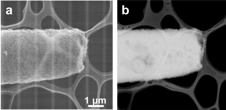
**Fig. 2** SEI-COMPO image (a) and CL image (b) of fluorescent material attached chitosan modified PLGA polymeric particles.
