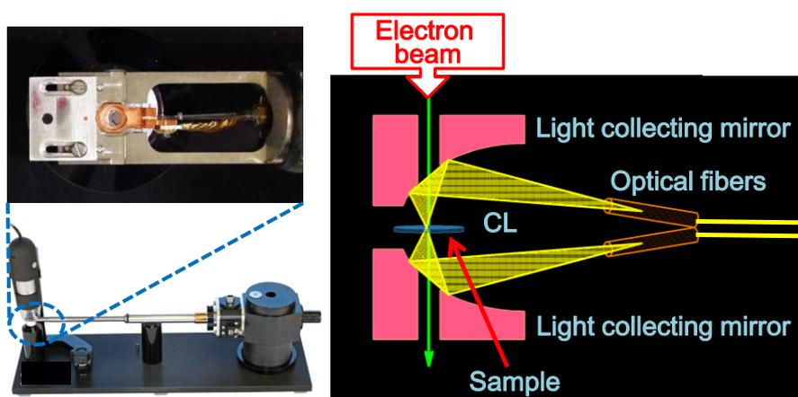
Fig. 1. Schematic image for the tip of the cryo holder and STEM-CL system.
