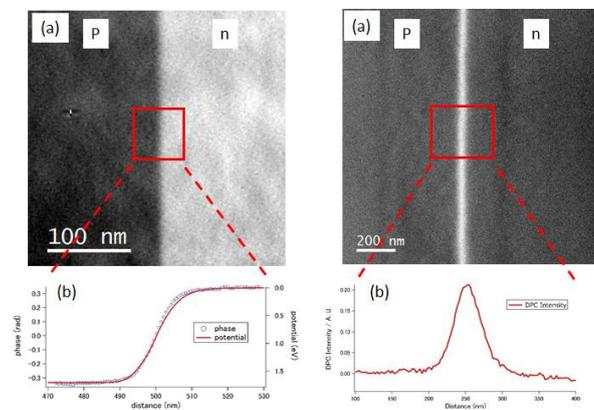
Fig. 1. Phase image and phase profile of p-n junction
