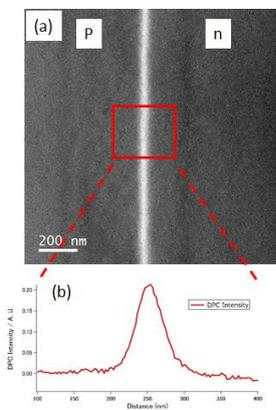
Fig. 2. DPC STEM image of GaAs p-n junction and intensity profile
