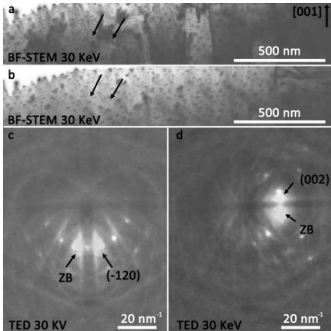
Fig. 1 (a,b) BF-STEM images and (c,d) corresponding TED patterns of InN. ZB indicates the zero-order beam.
