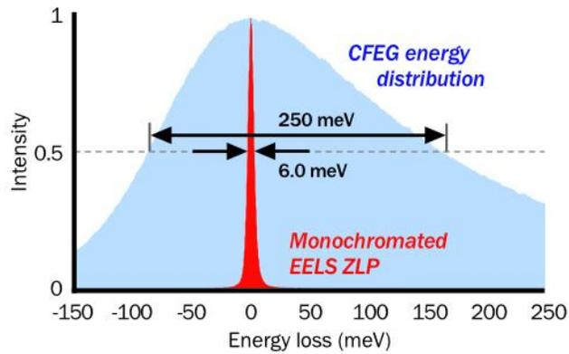
**Fig. 1.** Zero loss peak (ZLP) obtained at 60 keV primary energy with 100 ms acquisition time,  $\sim 11$  mrad half angle collection ( $\beta/2$ ) compared to unmonochromated CFEG energy distribution.
