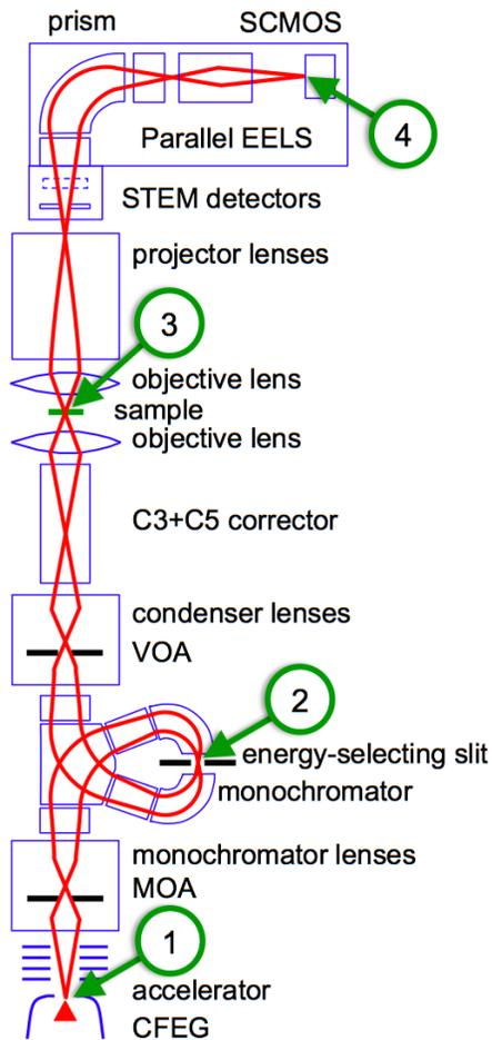
**Fig. 2.** Schematic diagram of the electron trajectories through the Nion ultra-high energy resolution monochromated EELS-STEM (U-HERMES). All the beam crossovers contain an image of the electron source; the most important crossovers are numbered: 1 = cold field emission gun (CFEG) virtual crossover; 2 = monochromator slit crossover; 3 = sample-level crossover; 4 = EEL spectrum crossover. (The trajectories are schematic and their widths are greatly exaggerated.)
