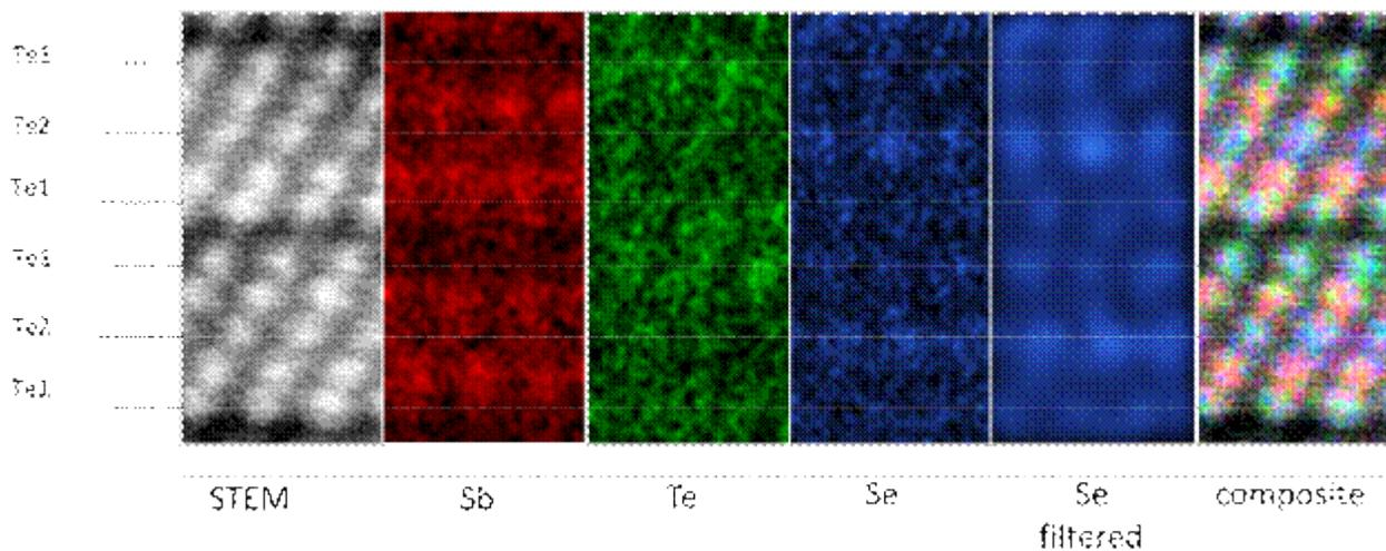
Figure 2. Atomic resolution STEM image together with elemental maps for Sb, Te and Se of  $\text{Sb}_2\text{Se}_{1.2}\text{Te}_{1.8}$  composition, showing Se atoms occupying preferentially Te2 positions.
