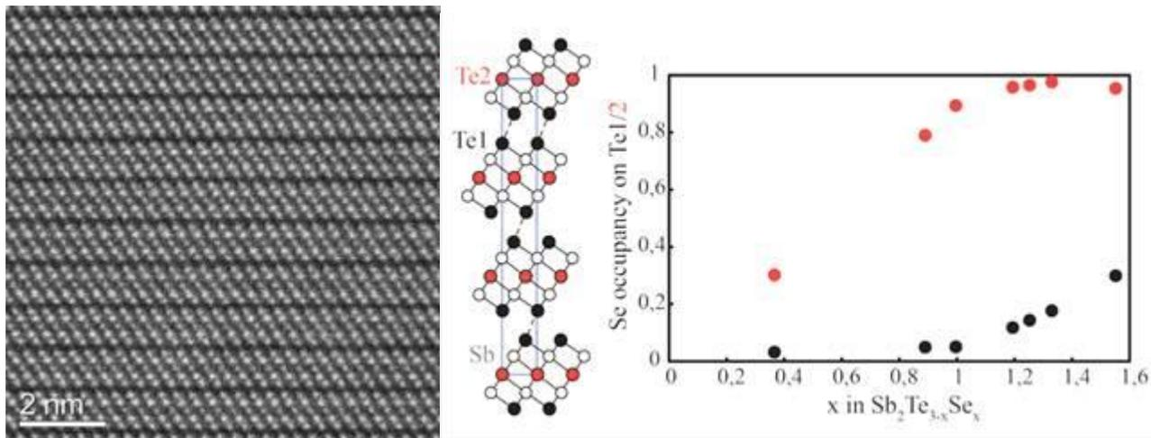
Figure 1. HR HAADF STEM image of  $\text{Sb}_2\text{Se}_{1.8}\text{Te}_{1.2}$  material, illustrating its layered structure,  $\text{Sb}_2\text{Te}_3$  structure model together graph showing the Se Te1/2 position occupation vs the Se concentration in  $\text{Sb}_2\text{Te}_{3-x}\text{Se}_x$ .
