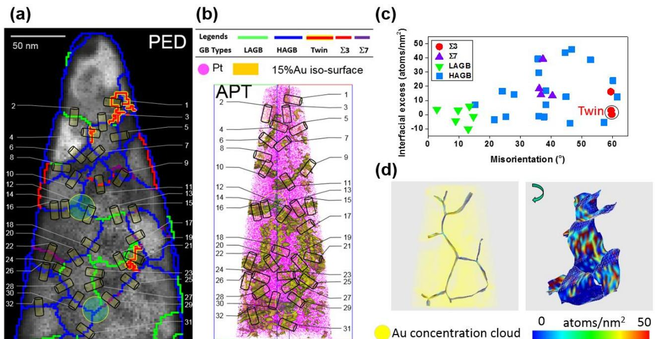
**Figure 1:** (a) PED map of the boundary segregation (b) APT reconstruction of (a) (c) IE values of different grain boundaries (d) visual IE map revealing variation of partitioning within the same boundary.
