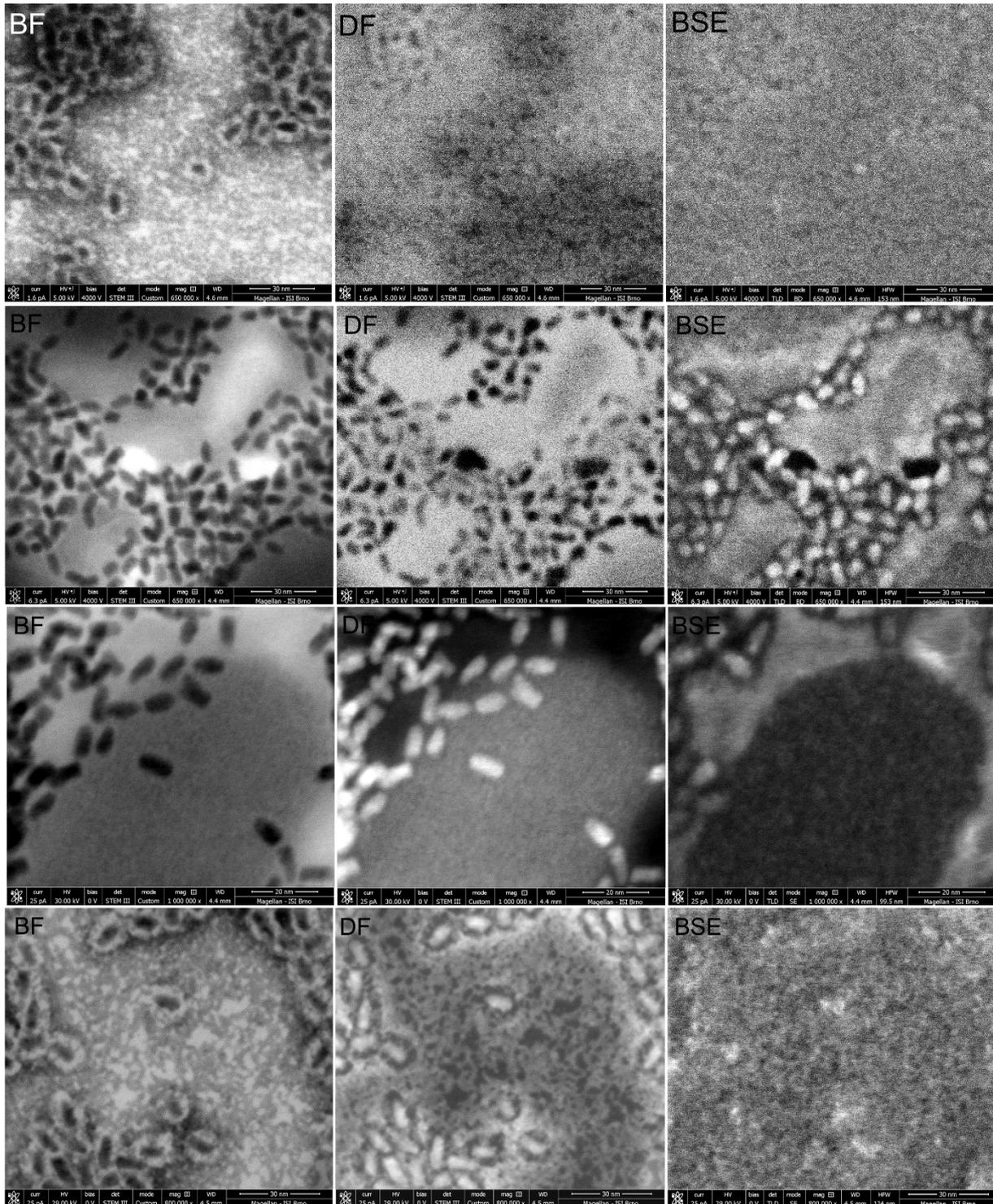
Fig.1. Images of Qdot™ 605 ITK™ Carboxyl Quantum Dots recorded on the stained/unstained sample at accelerating voltage of 5 keV and the sample potential -4 keV (the first/second row), on the unstained sample at 30 keV (the third row) and on the stained sample at 29 keV (the fourth row), both without any sample potential.
