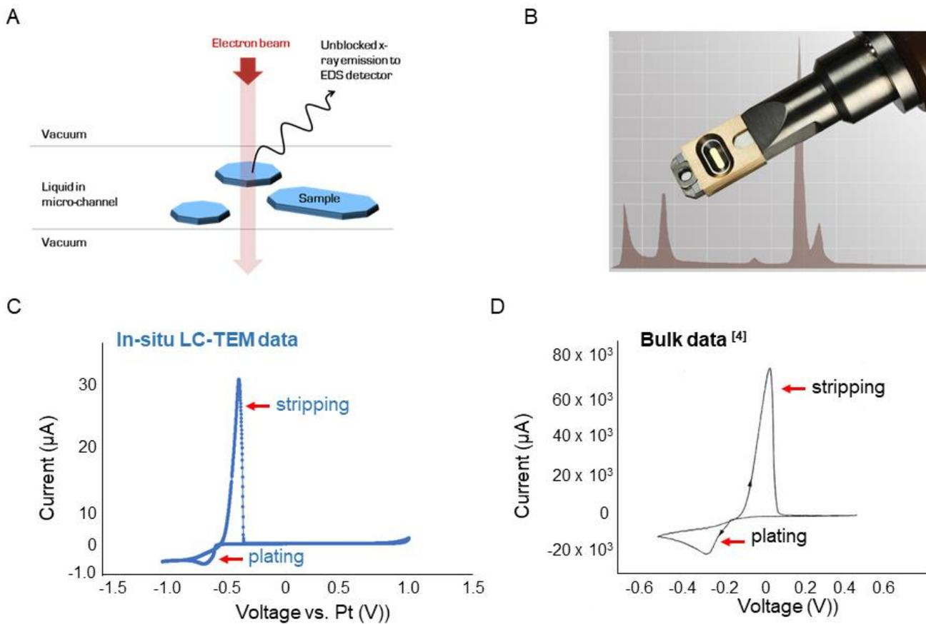
Figure 1. (A) Schematic of assembled liquid cell. (B) Liquid cell tip with EDS compatibility. (C) A CV curve of 0.1M  $\text{CuSO}_4$  performed in (C) in-situ LC-TEM, and (D) bulk cell extracted from Ref 4.
