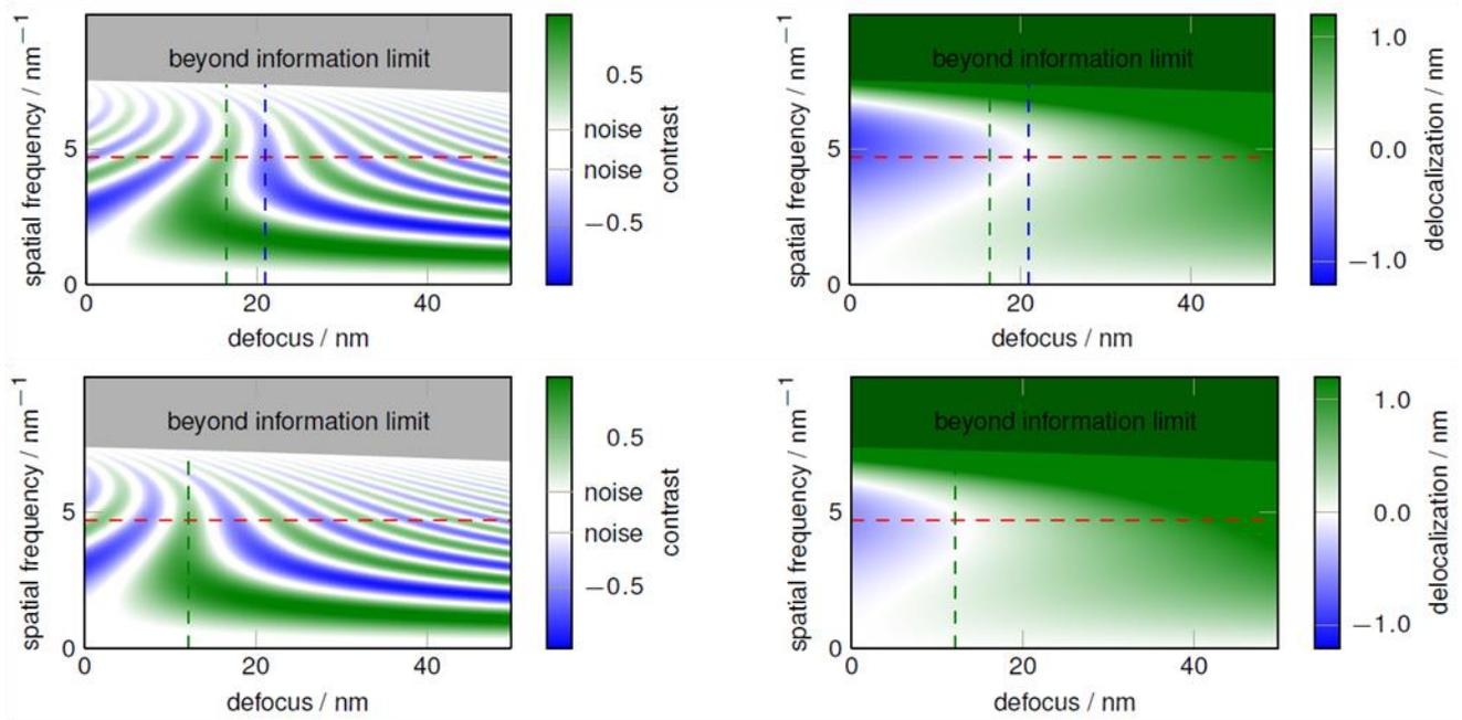
Figure 1. Phase contrast transfer and corresponding delocalisation in dependence of the defocus calculated for the SALVE instrument at 20 kV using *top* - Lentzen conditions (except the defocus) and *bottom* - depth-of-view optimised conditions.
