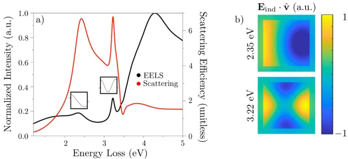
Figure 2: Simulated aloof EEL (black) and optical scattering (red) spectra of a 160 nm  $\text{CeO}_2$  nanocube. The electron beam is directed down the cube face in the aloof geometry and the plane-wave light field polarized normal to the cube face. The two insets display the electric field intensity profiles within the cube at the band-gap resonances. (b) The field maps show the electron-driven electric field distributions associated with the cavity modes at 2.37 eV (top) and 3.22 eV (bottom).
