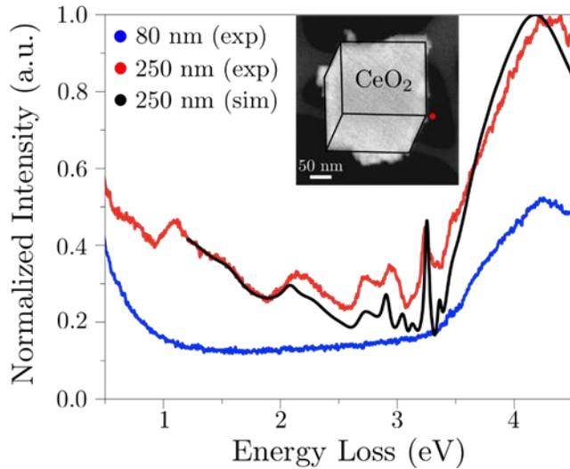
Figure 1: Experimental (red) and computed (black) aloof EEL spectra with the electron beam positioned 4 nm from the corner of a well-defined  $\text{CeO}_2$  cube of 250 nm in size. The aloof beam EEL spectrum (blue) from an isolated 80 nm  $\text{CeO}_2$  cube shows a featureless bandgap. The inset is the HAADF image of the 250 nm cube with beam position denoted by the red bullet.
