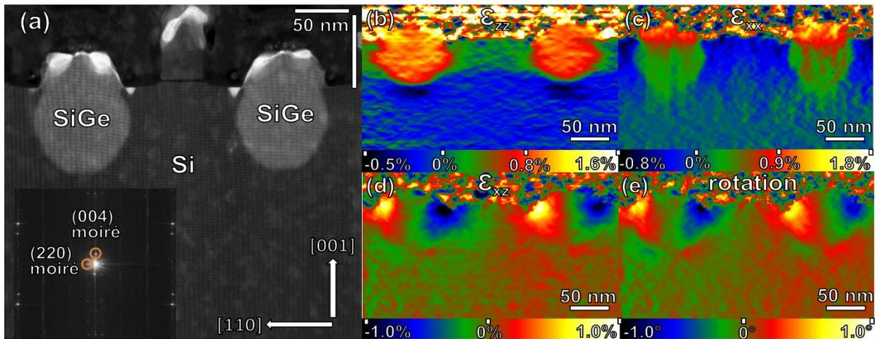
Figure 2: (a) 2D scanning Moiré pattern of a SiGe transistor in  $[110]$  ZA obtained by adapting the scan grid. (b)-(d) 2D strain components of the device retrieved from Moiré spacings using geometric phase analysis. The strain precision is around  $6 \cdot 10^{-4}$ .
