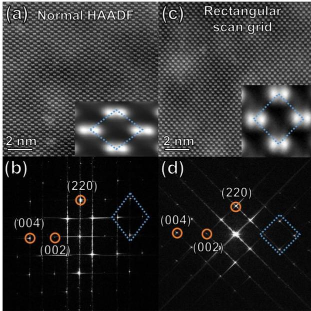
Figure 1: (a) HR-HAADF image of  $[110]$  Si with an enlarged view as inset and the corresponding power spectrum in (b). (c) Changing the scanning to make the scan grid rectangular results in a different image and the diffractogram (d) clearly shows the obtained square lattice from (220) and (002) planes.
