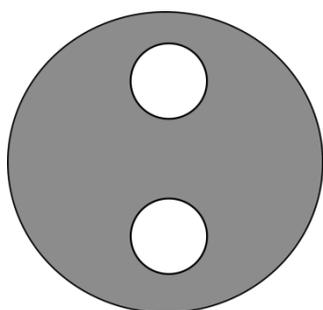
*Fig. 1. A schematic of DA strip, the white portions indicate the open areas*
