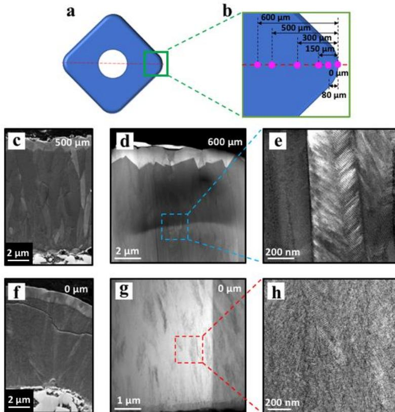
Figure 1: (a) Schematics of the CVD coated cutting tool. (b) Schematics of the area where the lift-out samples, the first from the edge corner (illustrated as 0 micron position) and the last from a position 600 micron away from it, are prepared. (c) and (f) SEM images of cross sections at 0 micron and 500 micron positions. (d), (e), (g) and (h) HAADF images of lift-out samples taken from 0 micron and 600 micron positions.
