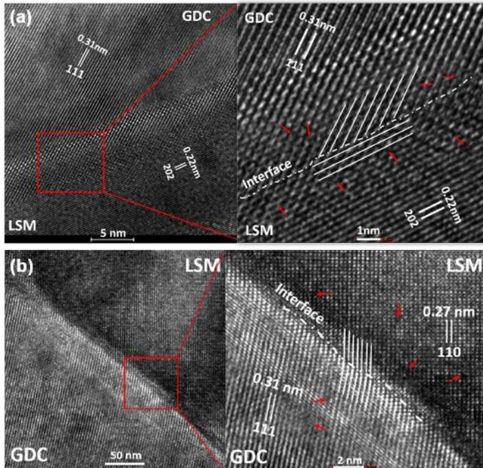
Figure 1. High resolution TEM of LSM/GDC interface induced by (a) high temperature sintering and (b) polarization.
